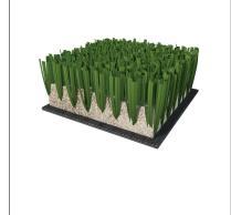
Latest generation artificial turf, manufactured with the TUFTING system. It has a gauge of 3/16" with 26 tufts/dm, resulting in 54.600 tufts/m². The STx available in different colors turf filament has a height of 12 mm and 9.000 Dtex.
