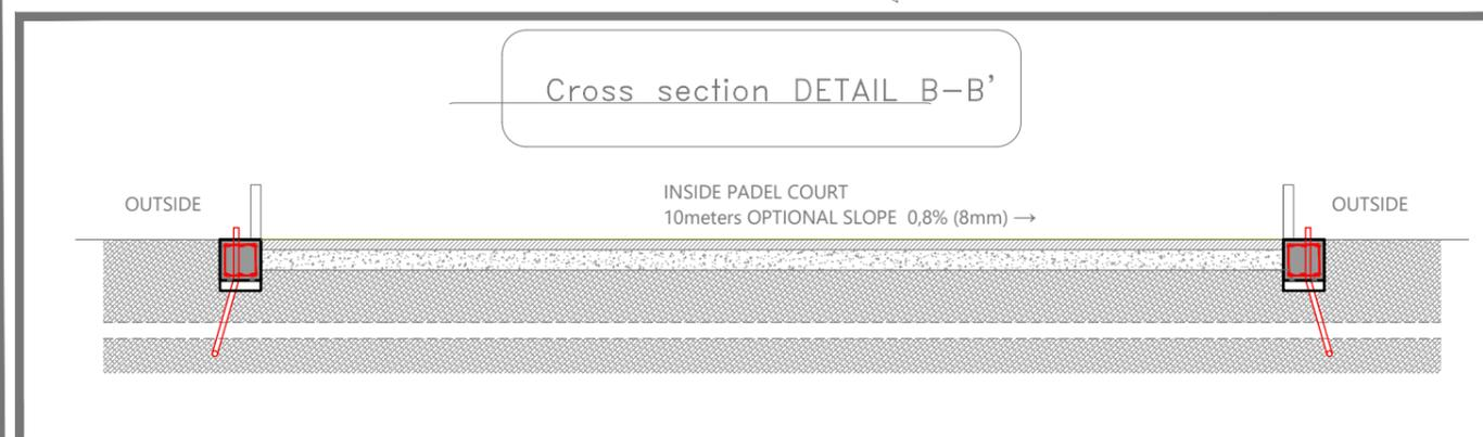
**NOTE:** The artificial turf carpet must be installed on a flat and if possible "rough" surface such as asphalt or unfinished cement. The following installation types must be avoided:
